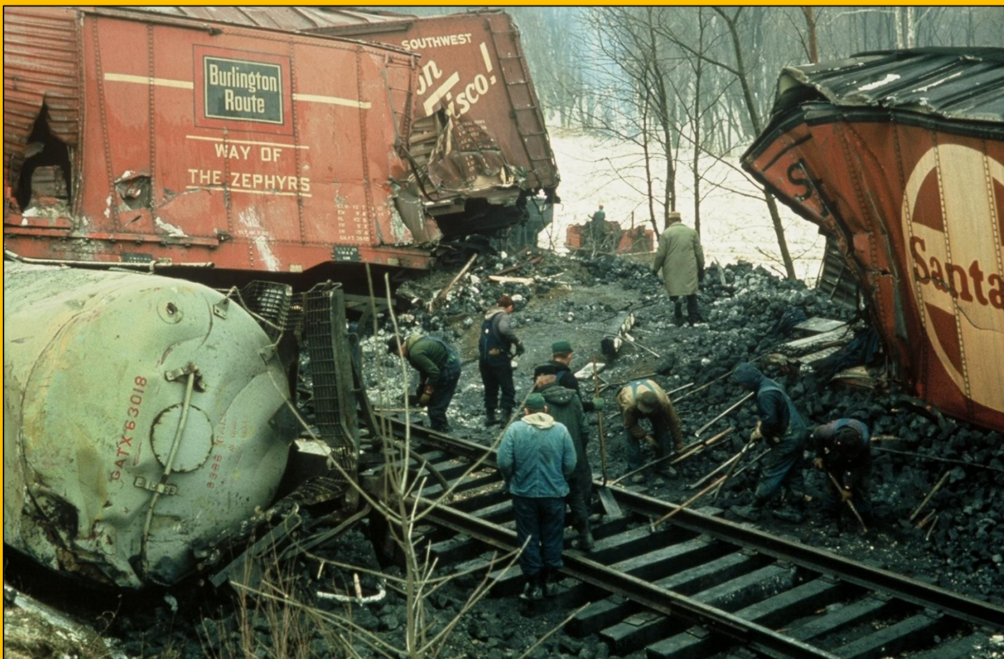
Above: A wreck occurred on February 4, 1966 near Tymochtee attributable to a broken rail, newly laid in 1964. No mention was made if Sperry Services had inspected this track segment. Jim Roberts, AC&Y HS Archive
