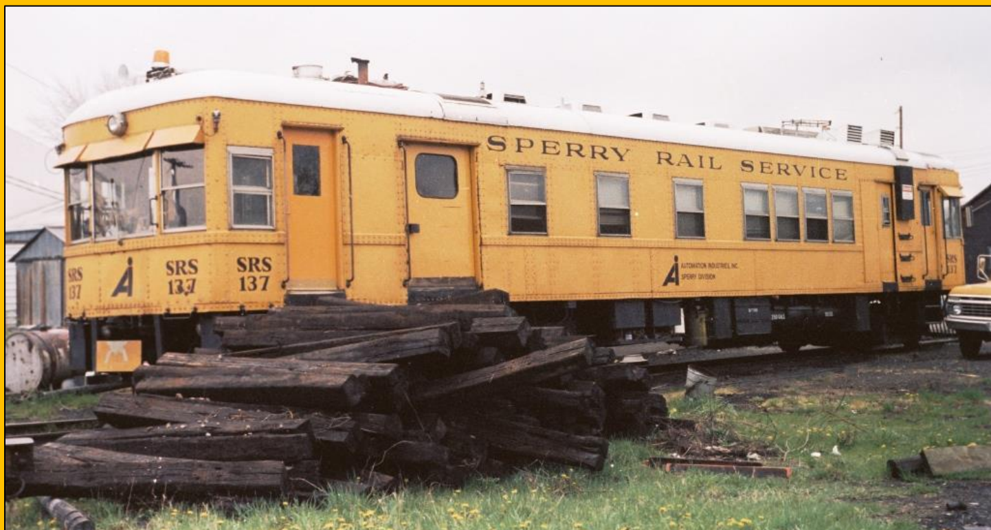
Above: Sperry Rail detection car number 137 is staged on the AC&Y at New London. The opposite side appears on the front cover. While water and power were self-contained, it likely was necessary to have a source of clean water and electrical hook-up at the end of each work day. At the detection speed of six-to-eight miles-per-hour, evaluation of the AC&Y's 169-mile mainline (Delphos to Brittain) would take twenty-four hours. It likely took three days. Vaughn Neel, AC&Y HS Archive
